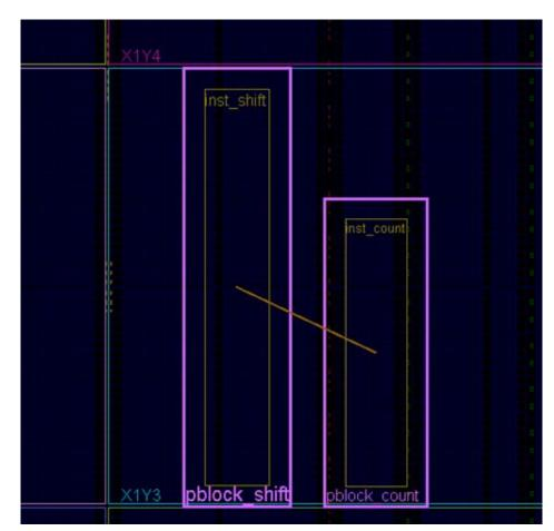
*Figure 3-2:* **RESET\_AFTER\_RECONFIG Compatible (Left) and Incompatible (Right) Pblocks**
