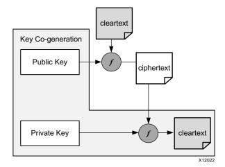
Figure 2-5: Asymmetric Key Encryption
