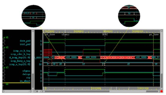
Figure 7-5: Vivado Logic Analyzer Display for Partial Reconfiguration
