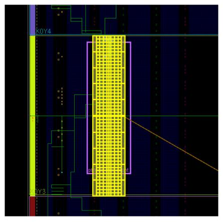
Figure 5-3: Original and Derived Pblocks using SNAPPING\_MODE
