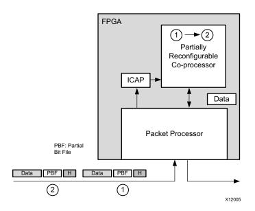
Figure 2-4: Dynamically Reconfigurable Packet Processor
