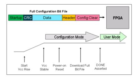
Figure 7-1: Configuring with a Full BIT File
