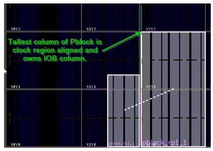
Figure 6-3: Tallest Column of Pblock Clock Region Aligned
