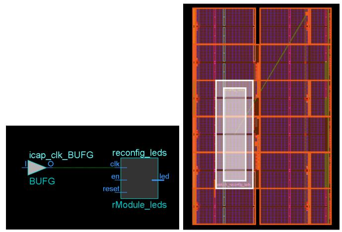
*Figure 5-1:* **Pre-routing Global Clock to Reconfigurable Partition**
