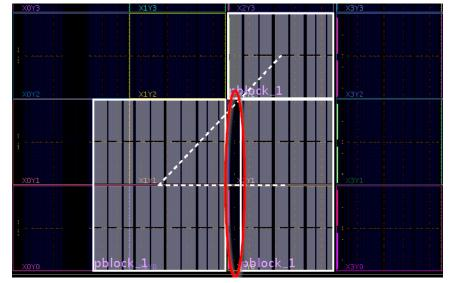
Figure 6-4: Gap in the IOB Column Not Supported
