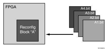
Figure 1-1: Basic Premise of Partial Reconfiguration
