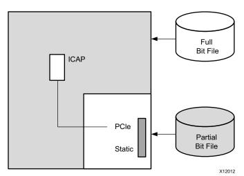
Figure 2-3: Configuration by Means of PCIe Interface
