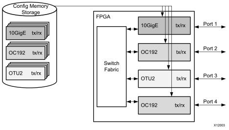
Figure 2-2: Network Switch With Partial Reconfiguration
