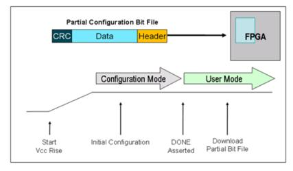
Figure 7-2: Configuring with a Partial BIT File
