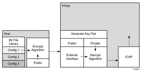
*Figure 2-6:* Loading an Encrypted Partial Bit File
