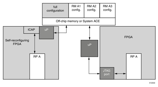
Figure 7-4: Configuring Through a Microprocessor
